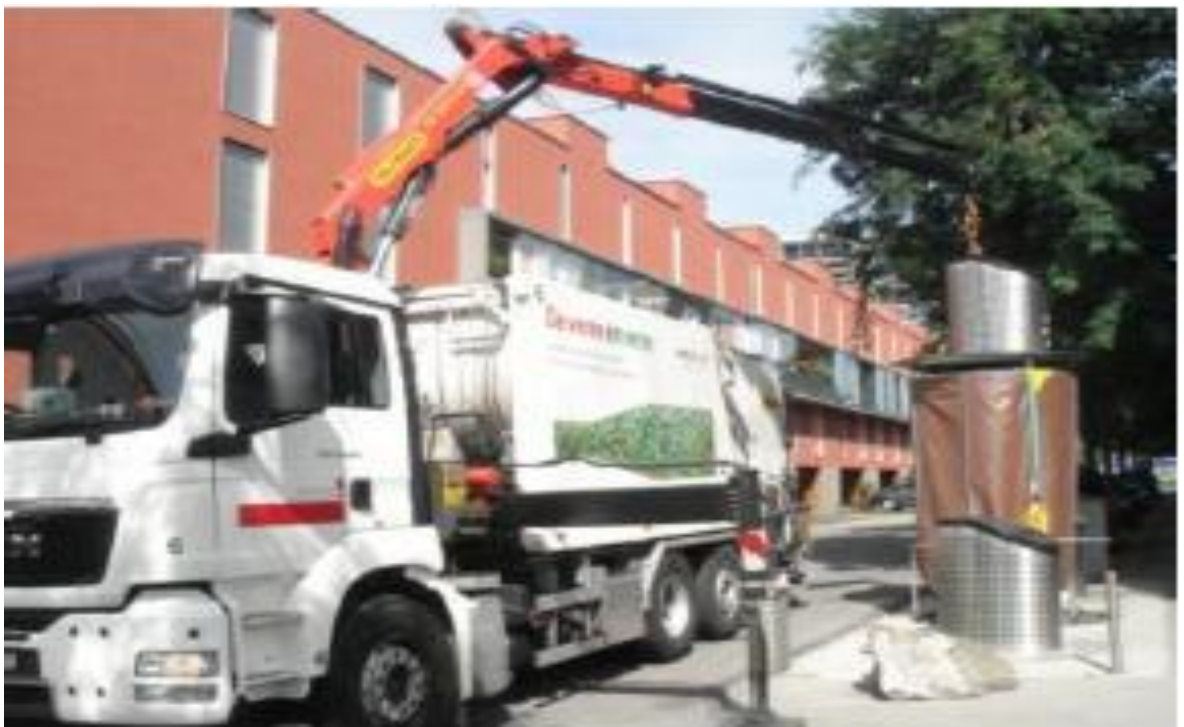
Figure 5-4 Loading and Unloading Mechanism of Semi underground bins
